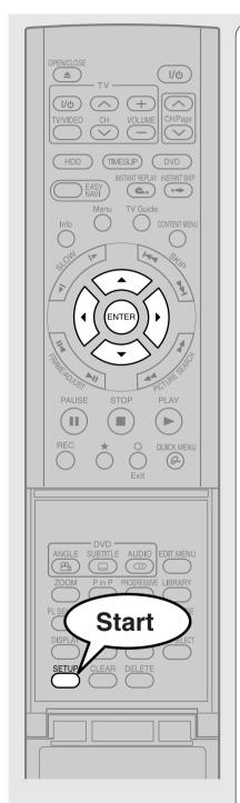
Press SETUP to display the setup menu.
